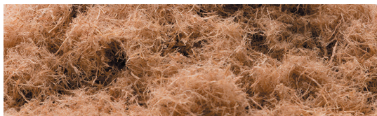
HydraFiber® is an approximately 98% porous fiber substrate with extremely low bulk density.
